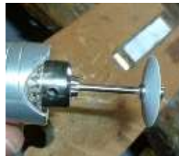
Mandrel placed off centre axis
